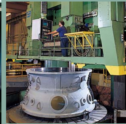
Schiess CNC vertical boring mill machining large turbine casing.
