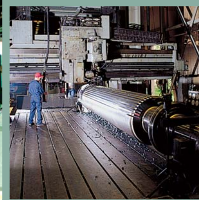
Large Ingersoll planer mill performing slotting work.
